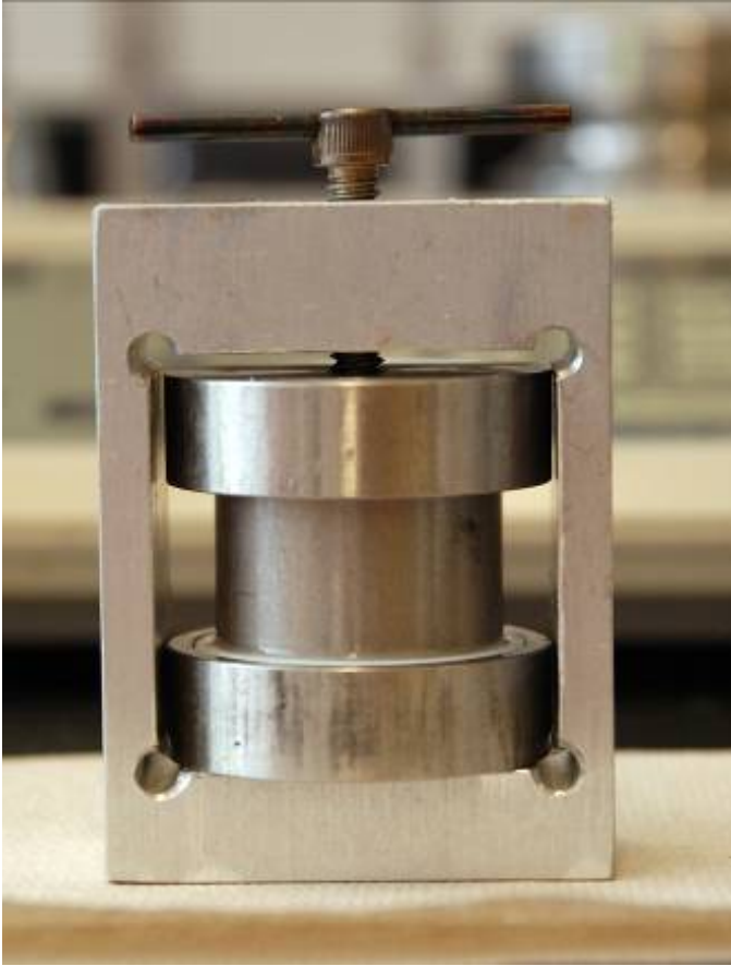
Figure 2 – Gel-forming device with clamp
